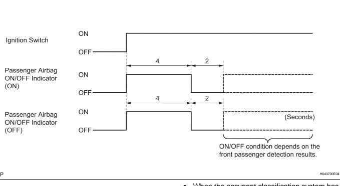
When the occupant classification system has trouble, both the SRS warning light and the passenger airbag ON/OFF indicator (OFF) come on. In this case, check the DTCs in the airbag system first.
